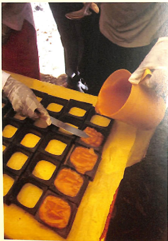
Plate 5. Pouring jelly-like soap into the moulds
